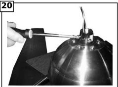
Loosen the 2 yoke screws.
